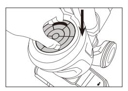
Replace HEPA filter by placing back on vacuum with the tabs facing up.
