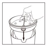
slot on front of dust cup and drop into position. Rotate handle down into position.
