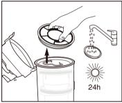
Lift out pre-motor filter and shake off dust frequently. Every three months, rinse filter and dry THOROUGHLY.
