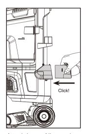
Attach hose. Align end of hose with inlet and push in. Clip will snap to secure in place.
