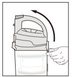
Pull dust cup latch to lift up dust cup lid.
