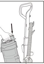
Press release button and lift off dust cup.
