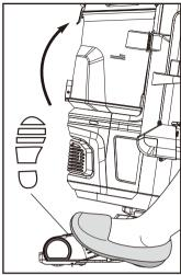
Step on nozzle and lower handle into position for vacuuming floors.
