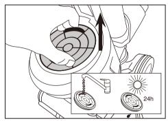
Grasp tabs on top of HEPA filter and lift it out of vacuum. **Note:** All filters are washable and can be cleaned by rinsing with warm water. Be sure the filter is THOROUGHLY dry before installing.
