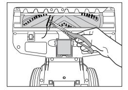
If brushroll stops spinning while vacuum is in use (not locked in upright position), this indicates the brushroll is cloqued and cannot turn. Brushroll will automatically shut off until clog is removed, vacuum is returned to its upright position and the handle is lowered again.
