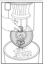
To empty debris, press lever to release bottom lid.
