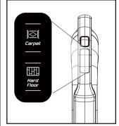
Press **FLOOR TYPE** button to choose between Carpet or Hard Floor mode. Icon will light up for selected floor mode.
