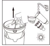
Rotate handle up to lift out filter screen. Tap to remove dust. Rinse dust cup and filter screen; dry THOROUGHLY.
