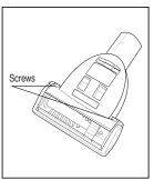
Turn nozzle onto back side. Remove 2 screws.
