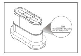
When the water in clean water tank is used up or the dirty water level reaches the Max line the suction drops obviously. Please clean it in time.
