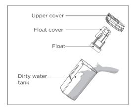
1. Remove the upper cover of dirty water tank, take out the float assembly
