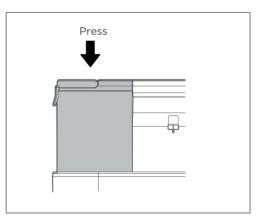
4. Reinstall the float back into the dirty water tank, buckle the upper cover and install them back to the machine and after hearing the click, the installation is successful.
