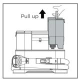
1. One hand on the machine, the other hand pulls clean water tank handle upward vertically, and the tank will be taken out.
