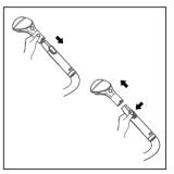
5. Insert the hose into the carpet brush. After hearing the click, the hose is successfully connected to the carpet brush. Press the lock cap, pull out in the direction shown in the picture, and then remove the carpet brush.
