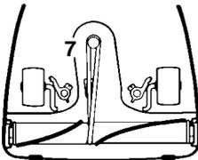
7. Place lower side of belt into belt guide and pull to stretch the belt around the left side of the motor pulley. Rotate pulley to secure belt into groove.
