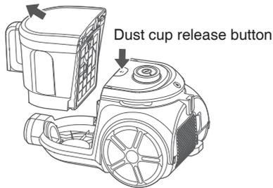
2. Remove the dust cup lid by locating the release button on the backside of the dust cup above the filter and press button up to pull lid off. Turn dust cup upside down to empty into trash bin.
