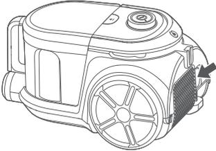
Remove the outlet HEPA filter from the machine.
