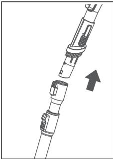
**Step 2:** Connect the telescoping metal wand to the hose
