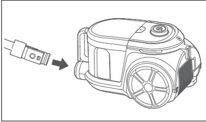
**Step 1:** Attach the hose to the front of the vacuum cleaner by inserting it into the air inlet until an audible click is heard.
