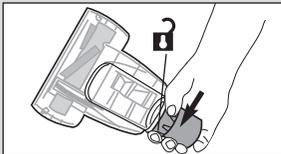
Grasp collar and twist counterclockwise to unlock cover. Lift cover up.
