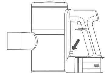
3. Rotate the motor cover component to remove the dust cup component.
