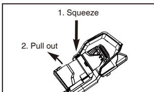
Press and squeeze-buttons, located on both sides at front of handle, at same time to release dust cup and pull dust cup out.
