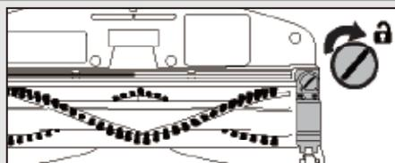
If debris cannot be removed easily, remove retainer clip to access brushroll. Using flathead screwdriver or coin, turn screw to the 'unlock' position.
