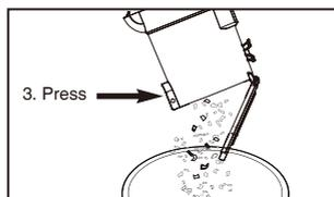
Press lever to release bottom lid of dust cup to empty debris.
