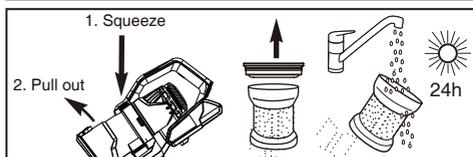
1. Press and squeeze buttons, located on both sides at front of handle, at same time to release dust cup and pull dust cup out.
