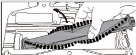
Remove retainer clip and lift out brushroll to clean and remove debris.
